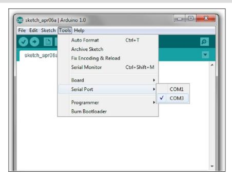
Double-click on the shortcut you made earlier to start the IDE. Go to Tools > Serial Port and select the COM port that the Arduino is connected to. (You can find out which one you're using by going back to the device manager.)
